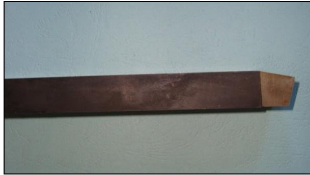
Figure 3 Cutting tool is medium carbon steel C.45 (water quenching)
