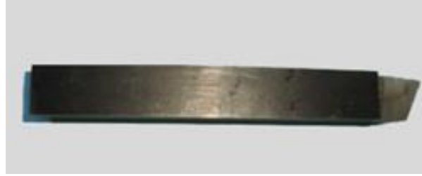
Figure 8 Cutting tool is medium carbon steel C.45 (oil quenching)
